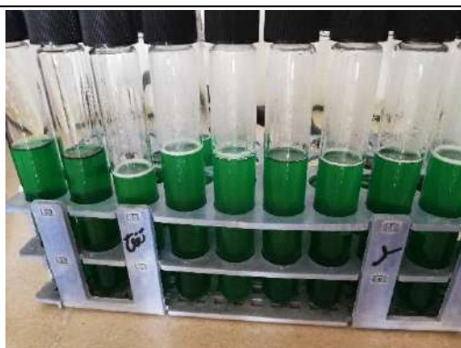
Multiple Tube Fermentation test via Brilliant Green Bile Lactose broth
